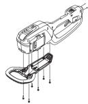
· Assemble the shock guard using the screws.
